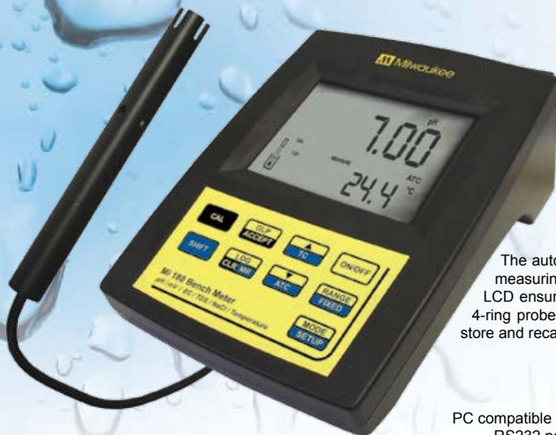
Mi180 measures 6 different parameters: pH, ORP, EC, TDS (Total Dissolved Solids), percentage of NaCl and temperature in a variety of ranges. pH calibration can be performed in 3 points selectable between 7 memorized buffers, to provide a very accurate calibration curve even when testing different samples, where very wide differences in pH can be found.
