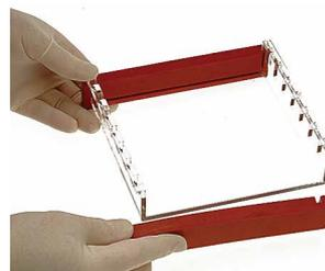
Casting dams allow gels to be rapidly cast externally while the unit is in use for gel running<sup>1</sup>
