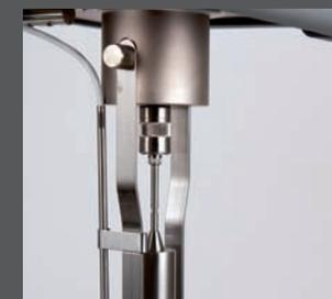
PT100 temperature probe is suitable adjusted by a clip which is attached to the spindle protector.
