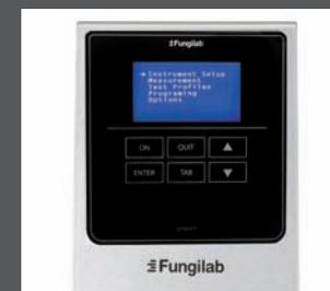
Front view of the viscometer, touch keyboard with 6 keys and graphic display.
