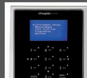
Front view of the viscometer, touch keyboard with 12 keys and graphic display.
