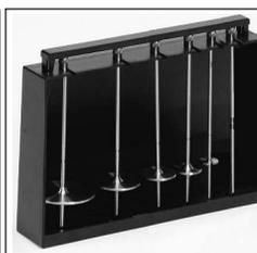
Rack of standard spindles R2, R3, R4, R5, R6 and R7: Suitable for model R.
