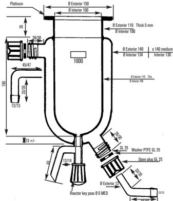
Reactor 0,5 liters. Part No. 1001960 Reactor 1 liters. Part No. 1001880 Part No. 1001879 Reactor 2 liters. Reactor 10 liters. Part No. 1001961
