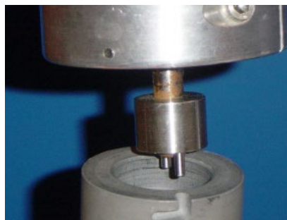
Figure 21. Coupling of motor and direct drive shaft
