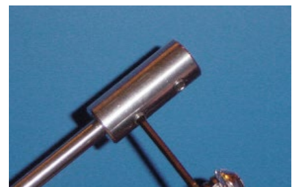
Figure 7. Tighten lower set screw (Step 5).
