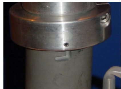
Figure 22. Correct orientation of motor on drive shaft
