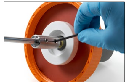
Figure 11. Tighten the upper set screw.
