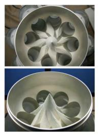
Powder with a high static charge or which is strongly adhesive should be fed through position B on the LABORETTE 27. (See  $\$  *Chapter 6.3 'Dividing suspensions and highly adhesive materials' on page 21*!)
